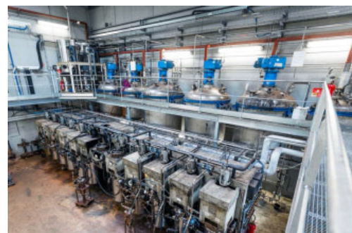
Figure 5 : Some of the emulsions are prepared in advance and stored in large tanks-agitators before use.
