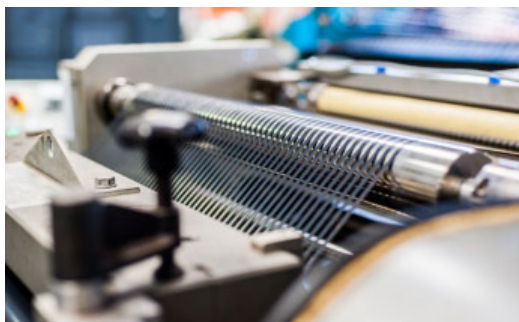
Figure 13: Slitting requires a very high precision to cut the rolls (jumbos) of coated film into tapes with a very accurate width
