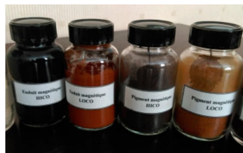
Figure 3 : Samples of magnetic pigments: low coercivity (LoCo) pigment is used for audio tapes
